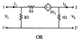
Determine the driving point impedance of the network given below.
